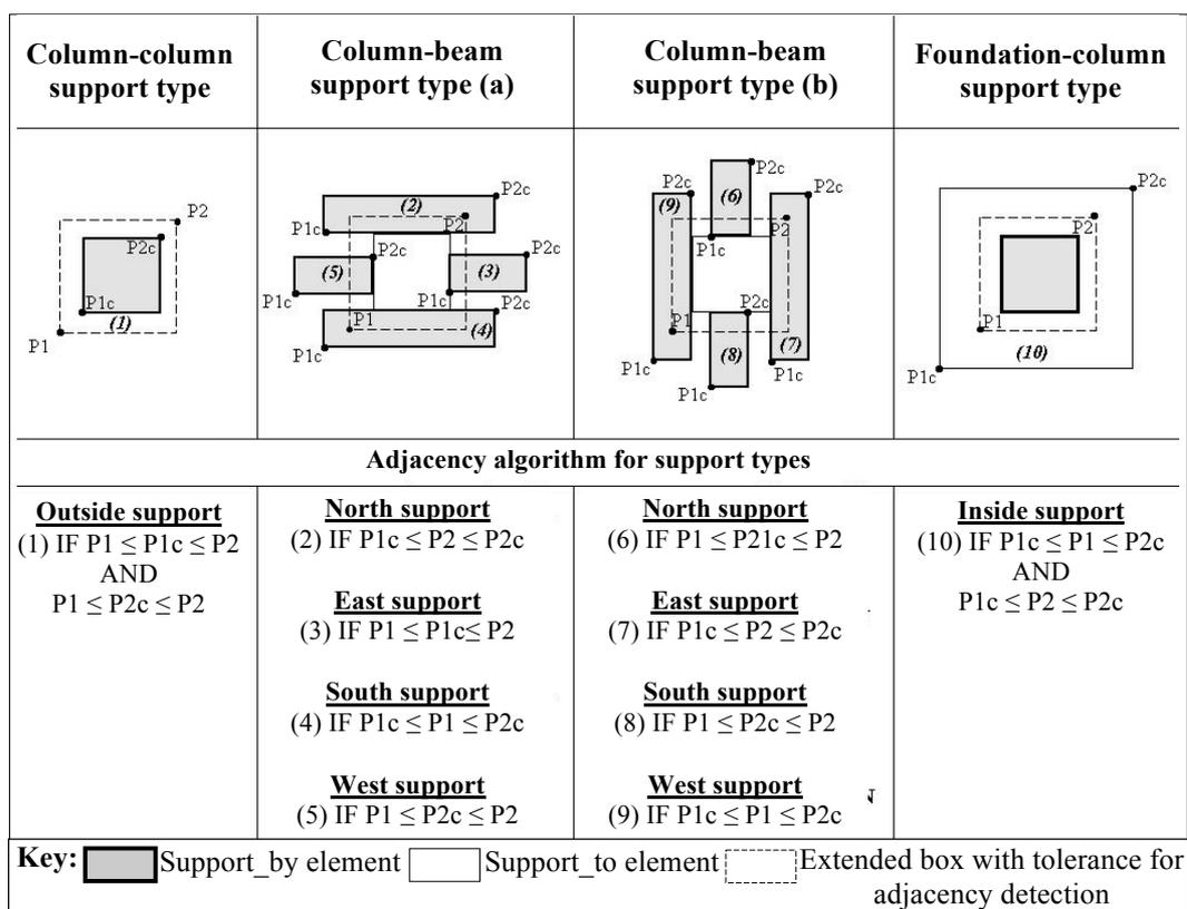
FIG. 5: Geometrical adjacency algorithm for ten support-to-support types
