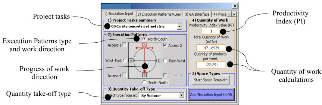
FIG. 4: Illustration of the Execution Patterns semantics in the developed 4D system interface
