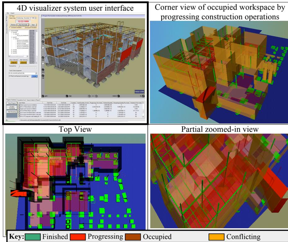
FIG. 13: Improving the construction workspace visualisation using VRML interface (source: www.iconviz.com)
