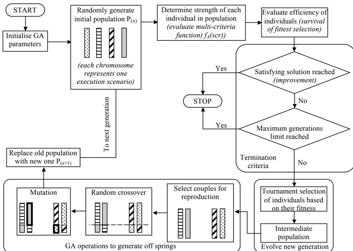
FIG. 2: Schematic of a Genetic Algorithms' evolutionary process
