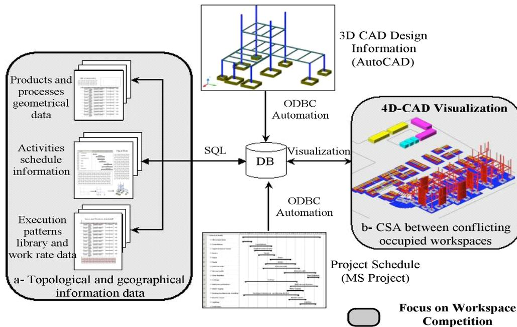
FIG. 1: Research focus using CAD systems for integrating design and construction information
