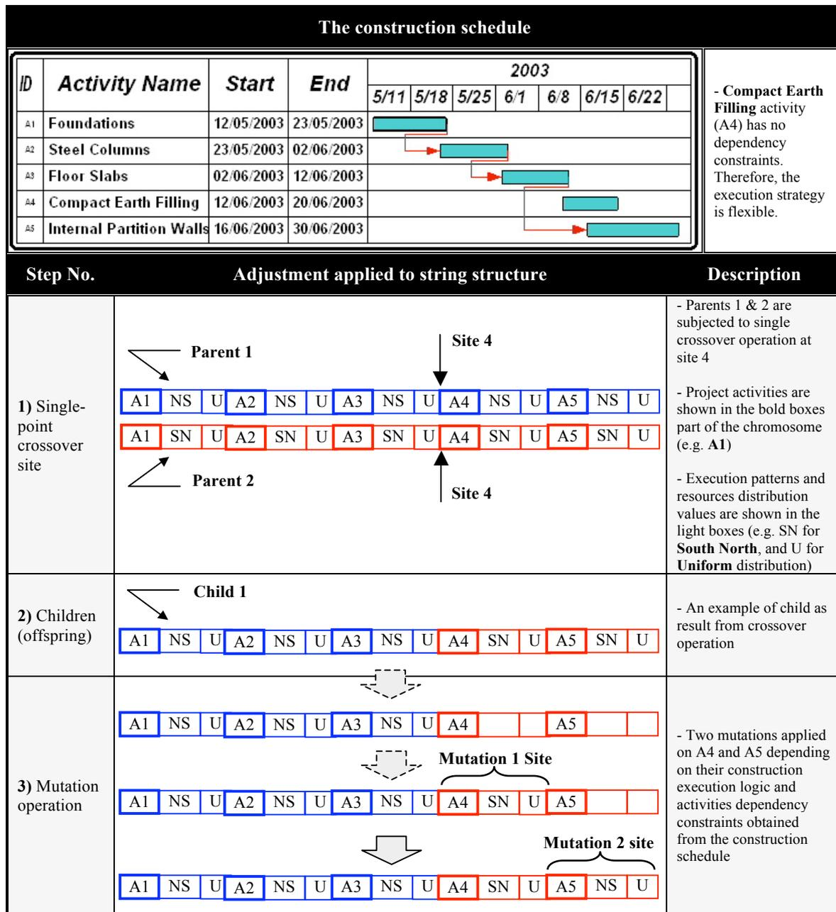
FIG. 6: Example chromosome structure, subjected to crossover and mutation operations
